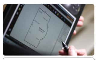
The intelligent drawing tool allows for easy input of room details and automatically calculates floor areas, subsequently populating this data into the site notes.
